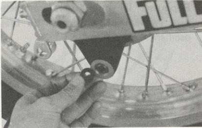
4. Spherical ball bearings and oil seals are used for this joint portion. Apply grease when installing the torque link.
