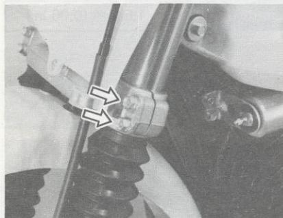
3. Loosen the clamp bolts. Pull down the front fork.
