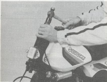
11. Draw out upper and lower bearing outer races by using special tool.
