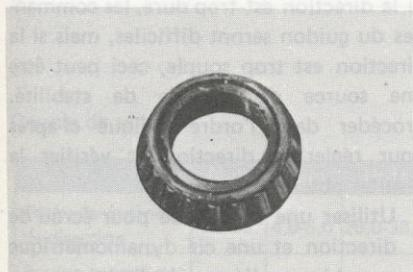
Apply grease upper ball bearings and lower bearing before remount the steering stem.
