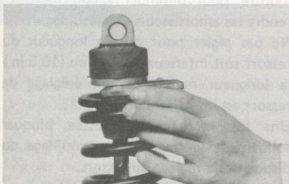
9. Special tool is available for removing and/or installing the optional springs.
