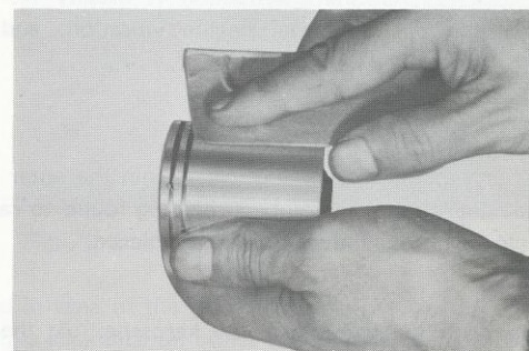
Fig. 65. Smoothing the sliding surface with emery paper
