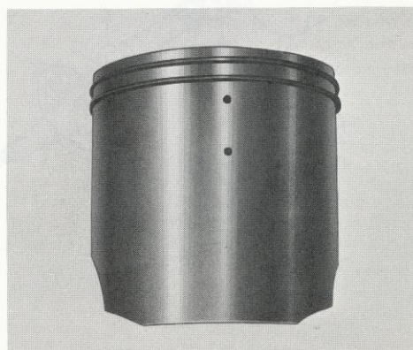
Fig. 5. Mixture bleeding holes in the piston wall
